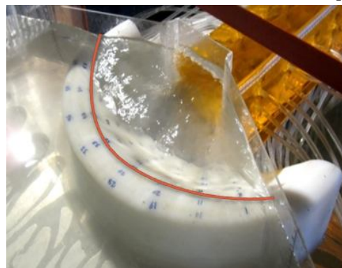
Figure 3- Formation of rooster tail in downstream of spillway
